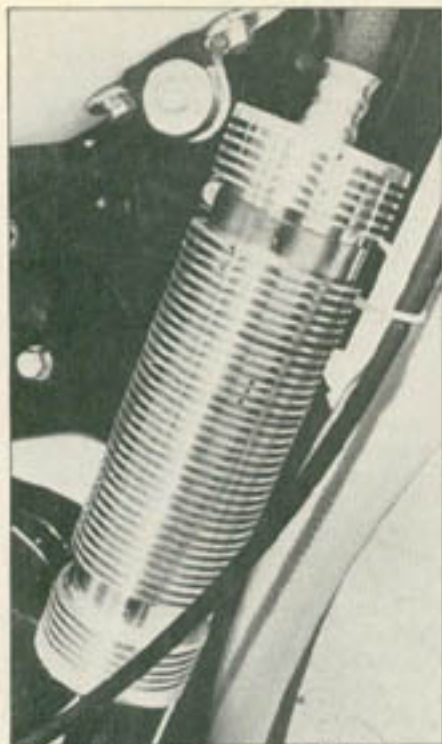
Luft's accessory reservoir is larger in volume and finned for increased cooling; the internal valving is also modified.
